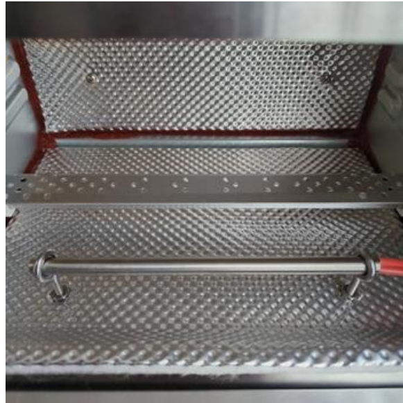
Adjusted Heater and Eye Bolts
